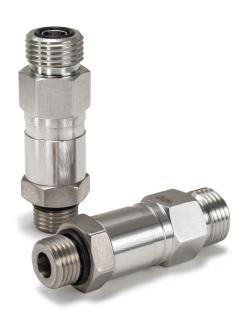
CVS Series check valves provide an important feature for CNG powered vehicles. When installed immediately after the fueling receptacle it functions as a redundant sealing device in the fill line, only allowing flow in one direction, from the dispenser to the vehicle.
