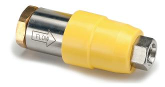
Parker's NGVBCN2-P50 fill line breakaway provides an important safety feature for CNG dispensing systems. It is certified to ANSI/NGV4.4/CSA12.54 standards for breakaway devices used on natural gas dispensing hoses and systems. It allows the hose to safely disconnect, preventing damage to the dispenser in the event of a "drive off" and sealing the CNG in the fill line to effectively prevent leakage or hose whip.
