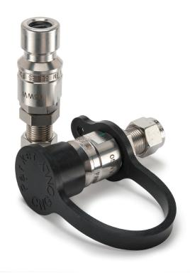
Parker FMS Series receptacles are designed for rigid mounting on a compressed natural gas vehicle. Receptacles can be employed in both fast-fill and time-fill dispensing applications. FMS Series receptacles are compatible with all CNG fueling nozzles conforming to the ANSI/NGV1 standards.
